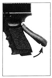
Remove the backstrap. This frees the loading port for the  $CO_2$  cartridge.
