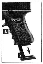
Press the magazine catch. Remove the magazine.
